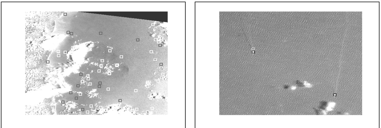
**Figure 2** The same scene as in Fig. 1 on another day with clouds and ocean wave. Right panel zooms in on an area with small clouds, waves, and two obvious ships. Ships are detected by various criteria discussed in the text. Ship wakes are a further confirmation that the detections are actual ships.
