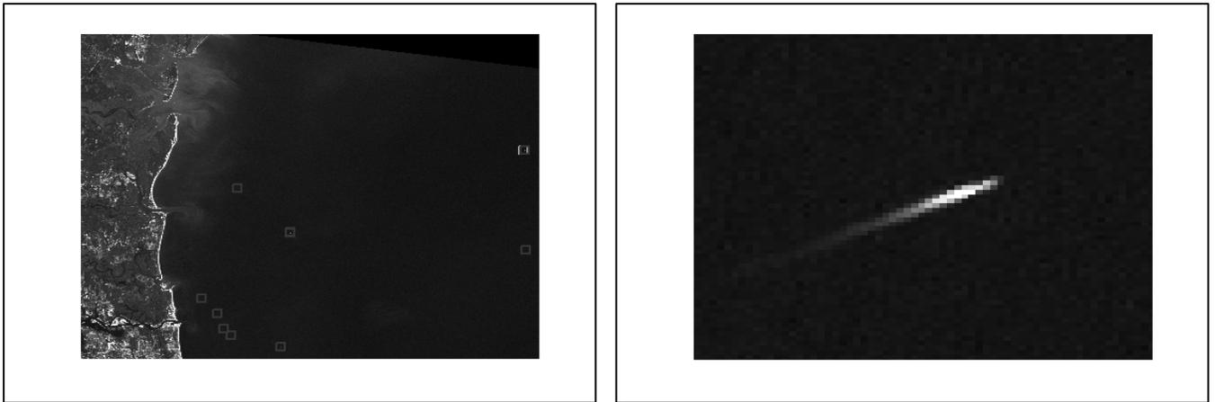
**Figure 1** A clear day image. Left: 100 km x 100 km area with squares marking candidate ships detected by automated processing; Right: zoom-in on one of the candidates showing a bright ship hull and trailing wake.
